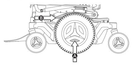
The serial number label is located on the lower, left side of the wheelchair chassis. Look between the rim spokes **a**. An additional serial number label is located on the seat tilt **b**. You may need to tilt the seat for better visibility.
