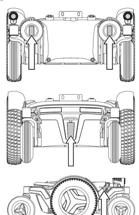
The wheelchair is equipped with reflectors at the front, the rear, and the sides.
