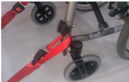
Fitting the Front Restraint
