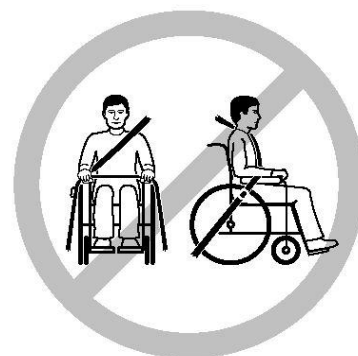
Incorrect seat belt position
